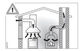
Great care should be taken when using the cooker hood at the same time and in the same room or area of the house as another heating appliance which depends on the air in the room. Such appliances include gas, oil, wood or coal-fired boilers and heaters, continuous flow or other water heaters, gas hobs, cookers or ovens which draw air in from the room and duct exhaust gases out through a chimney or extraction ducting.
